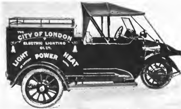
Three-wheeled Torpedo electric, with van body, used in London. The driver is protected by the top and windshield
